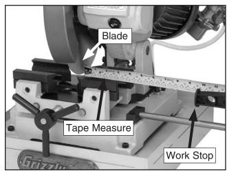
Figure 13. Measuring length of cut.
